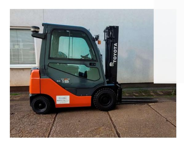
For material handling, an additional forklift Toyota 02-8FDF18 with diesel engine was purchased. It has a lifting capacity of 1750 kg and is equipped with a lifting device in duplex version with a height of 3300 mm. The equipment of this lift includes pneumatic tyres which absorb shocks and therefore the movement is possible even on uneven surface.
