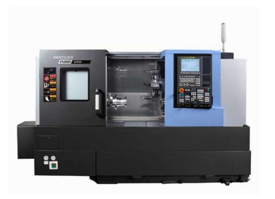
The company purchased a Doosan Puma GT high-precision horizontal lathe. The lathe has a 600 mm over bed diameter, a maximum turning diameter of 390 mm, a maximum turning length of 562 mm, 4500 rpm and a tool count of 12 tools in the automatic tool head.
