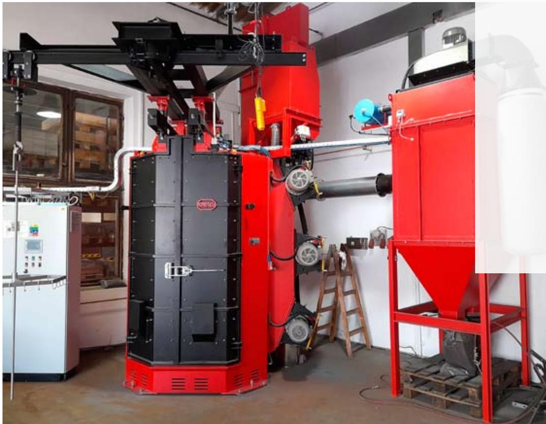
In 2022, the Optima New blast machine with blast wheels was purchased. The equipment is designed for blasting parts suspended on rotating and moving hook. The abrasive is thrown onto the rotating and moving parts at the same time from below and above, thereby striking the entire surface of the part in one blast cycle.
